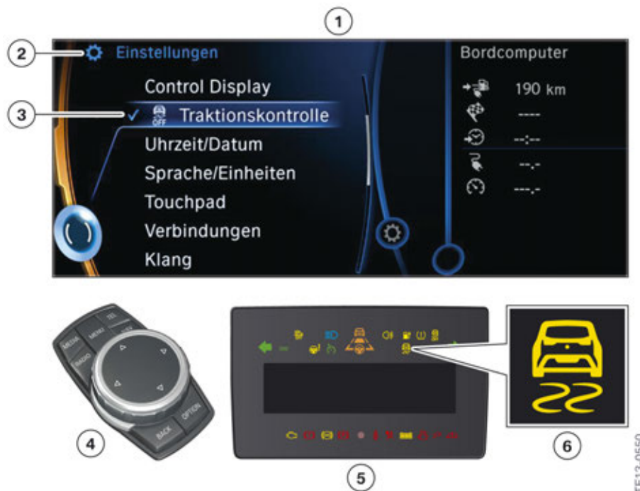
Activation of the DTC in the I01
