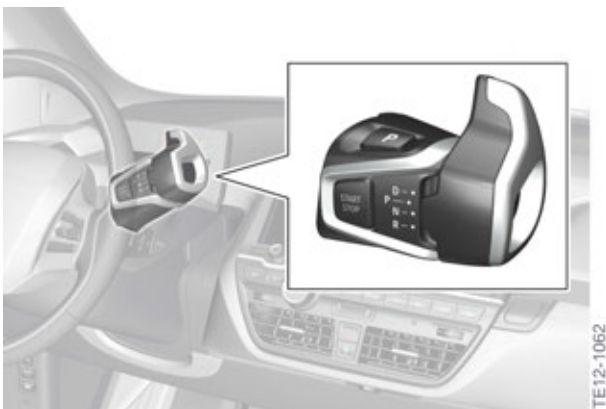
Installation location of the gear selector switch in the I01
