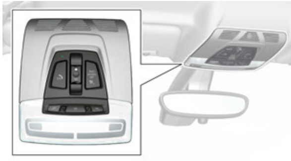
I01 Roof function center with indicator lamp for front passenger airbag deactivation
